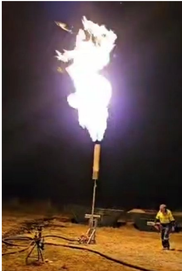
Figure 1: Production Test Well 271-KA03PT06 being choke tested
